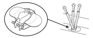
Fit the new strain relief device to the mounting bracket by removing the two clamping screws, feeding the two halves (ears first) through the hole in the mounting bracket and loosely refitting the screws. Insert the power cord through the strain relief device but do not tighten the device yet.
